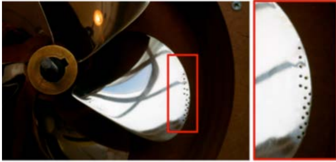
Figure 6. Applying holes on the propeller of the ship [21]
